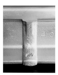
A modification of the process was introduced in 1995 which incorporated a second riser on each side of the foot, positioned between the normal riser and the foot tip. This type of weld is referred to as the SkV-F+ weld. Welds of this type will only be found in BS 113A or BS 110A rail, or equivalent profiles.
