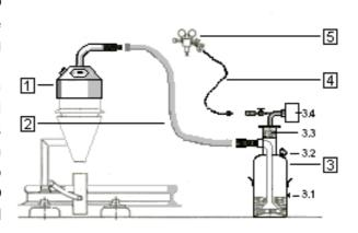
suction hood is fabricated with an outlet pipe for connection to the filter unit via a flexible steel hose (2).
